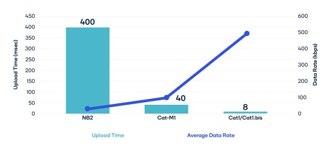
Figure 1: Device ON time for NB2, Cat-M1 and Cat 1 devices
