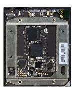
The Snapdragon 845 Processor Card measuring 60mm x 70mm is where all the processing occurs. It is connected to the carrier via two 240-pin high speed board-to-board connectors. A top side heat sink and a bottom side heat conductive metal plate provide thermal protection.
