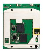
The Snapdragon 835 Processor Card measuring 60mm x 70mm is where all the processing occurs. It is connected to the carrier via two 240-pin high speed board-toboard connectors. A top side heat sink and a bottom side heat conductive metal plate provide thermal protection.
