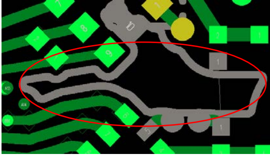
Figure 3-1 Example: ground plane without ground vias
