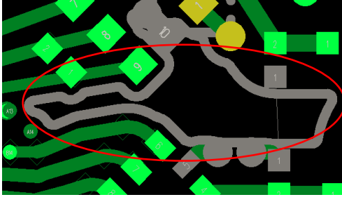
Figure 2-13 Ground plane without ground vias
