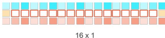
**Figure 9-10 Process 16x1 pixels: load 18x3 pixels**
